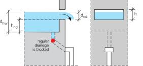
NL2.10 Dimensions of an emergency drain for a flat roof with a straight free overfal.
