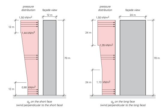
NL2.16 Distribution of the peak velocity pressure qp(ze) over the height of the short and long faces.
