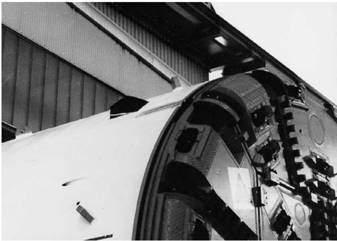
Figure 10-8 Stabilising shoe shield TBM S-160 (Herrenknecht), Metro Porto, \varnothing 8.7 m, 1999 [61]
