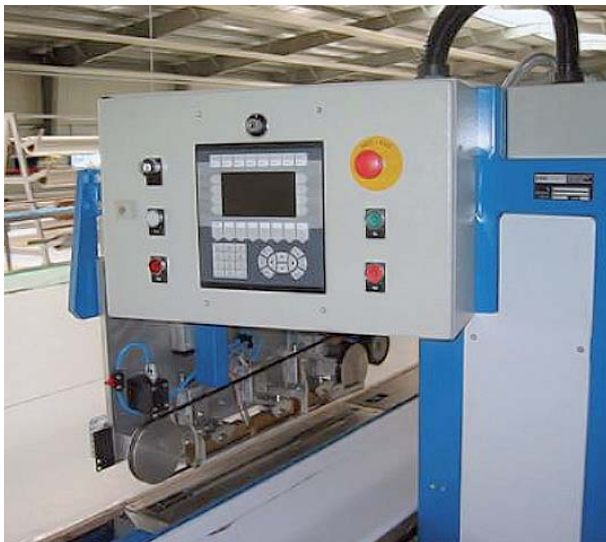
Fig. 116: Welding of ETFE foils
