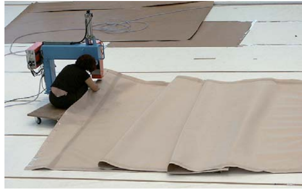
Fig. 119: left: PES/PVC fabric corners of a circus tent reinforced with sewn seams; right: Sewing the edge area of a Glass/PTFE fabric
