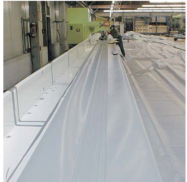
Fig. 114: Welding under pretension
