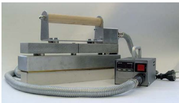
Fig. 117: left: Manual welding device; right: Mobile magnetic welding device
