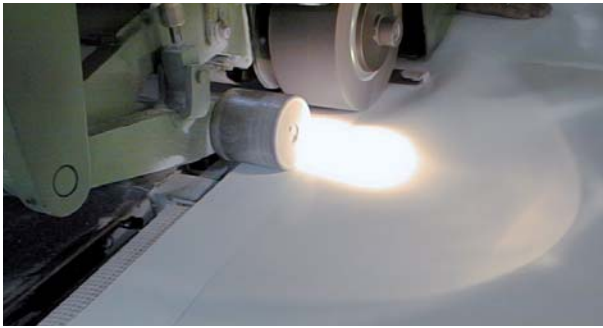
Fig. 112: Grinding off the PVDF paint
