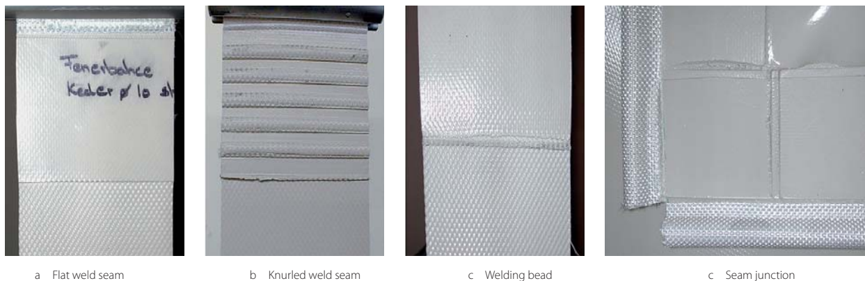
Fig. 111: HF seam types
