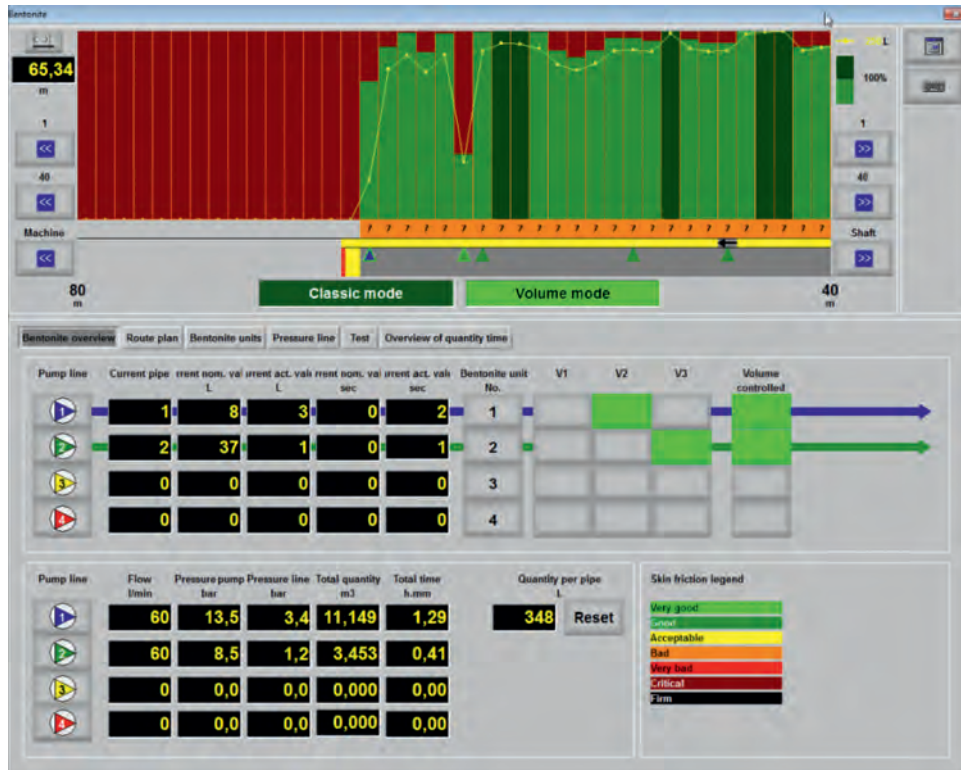
Fig. 7.32 Display of the system monitor of a volume-controlled lubrication system. (Source: Herrenknecht AG).
