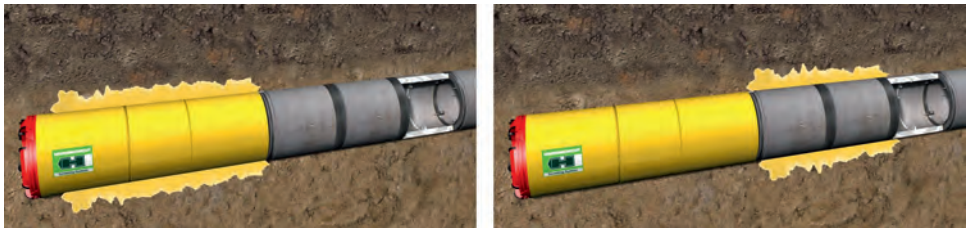
Fig. 7.34 Transfer of the initial injection: left normal initial injection, right initial injection in case of great danger of the shield rolling. (Source: Herrenknecht AG).
