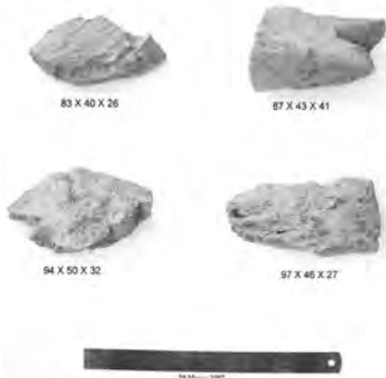
b) Muck size in fractured zone
