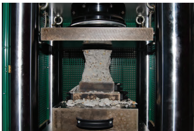
Figure 4.9 Testing apparatus in which concrete cubes are loaded to failure (photo: Kuhn).
