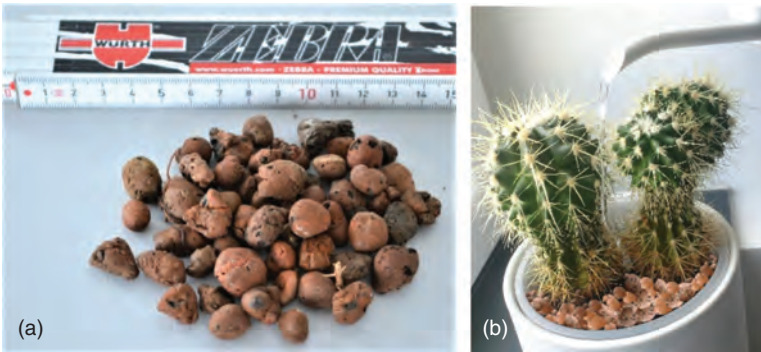
Figure 4.6 Aggregate for lightweight concrete: expanded clay pellets, (a) expanded clay or expanded slate, (b) hydroponic plant (photos: Scheller).
