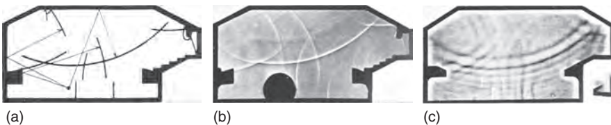
Figure 26.9 The progress of ripples in a sectional model of an auditorium. (a) Geometric construction. (b) Sound pulse image. (c) Ripple tank image. (Source: [5] Plate VII)
