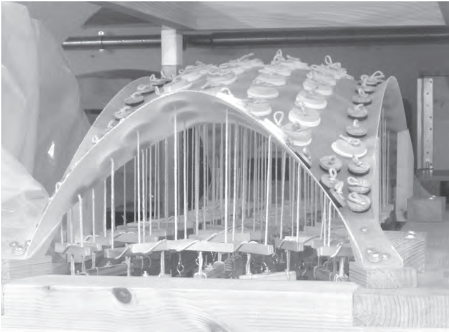
Figure 39.7 Model of one of Heinz Isler's characteristic shell roofs in its original testing apparatus. Now located in the Isler Archive at the ETH, Zurich. (Image: Bill Addis)
