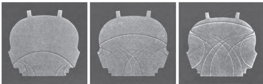
Figure 26.1 Sound-pulse photographs by Sabine showing the progress of a single wave through a plan of a theatre. (Source: [4] Figures 22-24)
