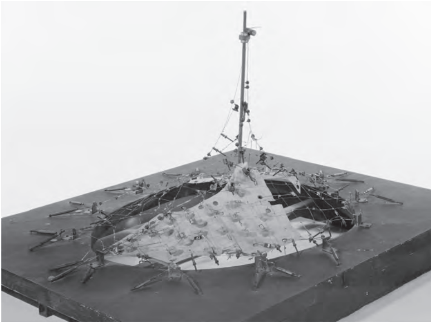
Figure 39.8 Measurement model of Frei Otto's IL Pavilion at the University of Stuttgart. (Image: Architekturmuseum München)
