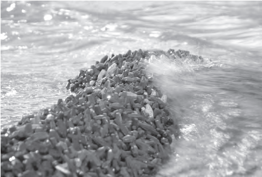
Figure 31.2 Waves breaking on a physical 1:48 scale model of a breakwater. (Image: © HR Wallingford)
