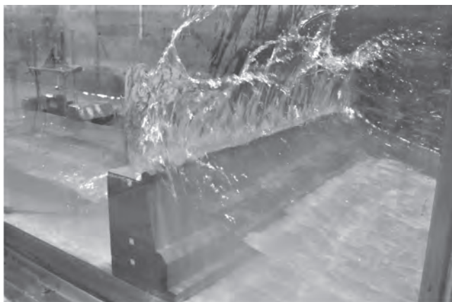
Figure 31.1 A 1:30 scale model test showing wave overtopping of a seawall. (Image: © HR Wallingford)
