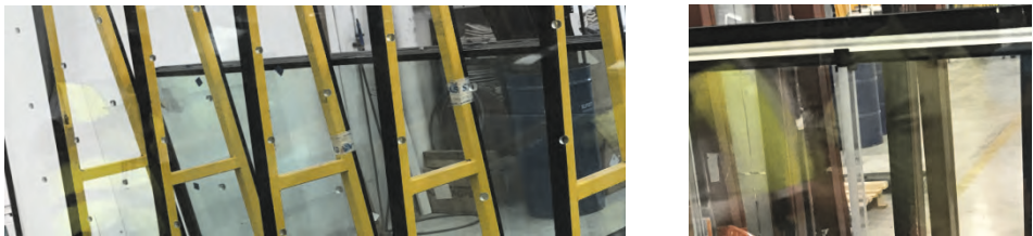
Figure 2-3 Prototypes for punctual (left) and linear (right) bracing components in the cavity.
