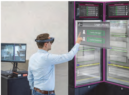
Figure 3-2 Interaction between users and facades by means of AR-Glasses and edge computing. (© Peter Neusser. seele)
